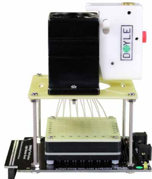
Side View Showing Fibers Entering Mating Connector
